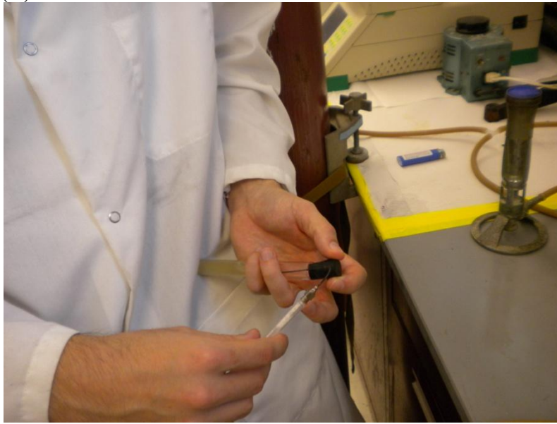
Fig. 3. Placement of substrate tube in clamp. Feeding pipette and gassing probe also in place.
