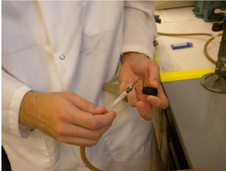
Fig. 2. Method of holding culture tubes, stopper, and gassing probe. (A) Position for opening tube. Needle is held near lip of culture tube for immediate insertion after stopper is removed. (B) Position for holding open tube for feeding and other manipulation. (C) Position for stoppering tube. Needle is kept between wall of tube and stopper, and needle is slid out as stopper is slid in.
