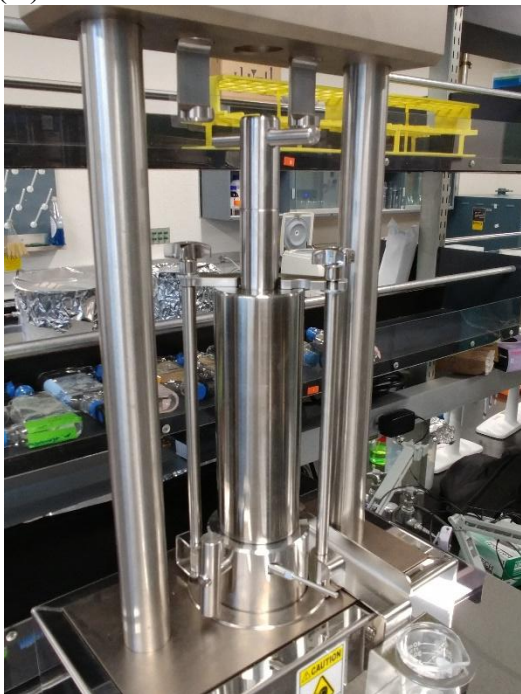
Fig. 5. Operation of cell press. (A) Before operation. Cell body and lower platen are in fully lowered position. (B) During operation. Cell body and lower platen are in intermediate position. Piston has made contact with upper platen. (C) At end of operation. Cell body and lower platen are in fully raised position. The STOP line on piston has been reached. (D) Close up of STOP line in (C).
