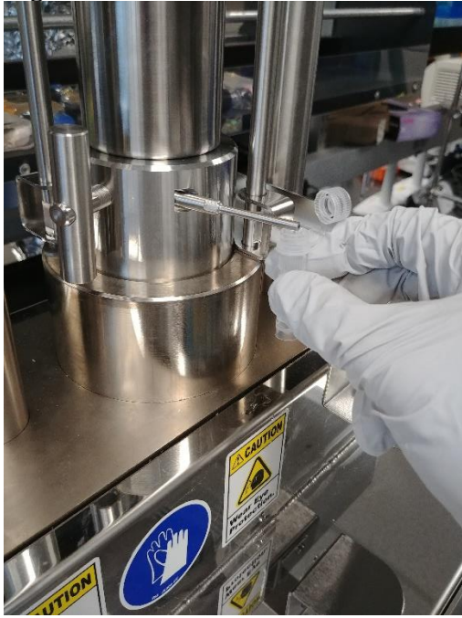
Fig. 6. Collection of cell extract in centrifuge tube.
