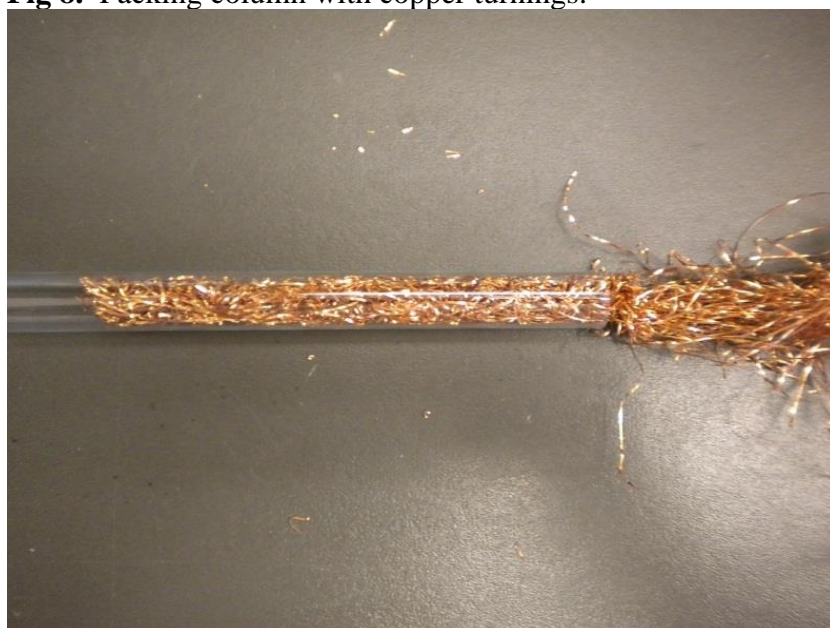
Fig 8. Packing column with copper turnings.
