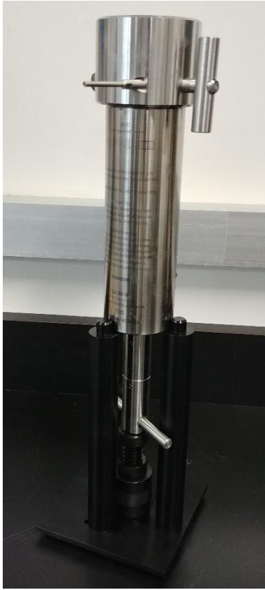
Fig. 2. Pressure cell assembled and loaded on stand
