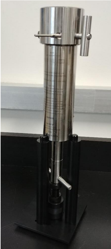
Fig. 2. Pressure cell assembled and loaded on stand
