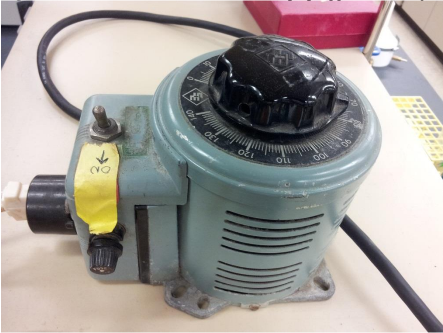
Fig. 14. Rheostat (140 V, 10A), with heat tape plugged in and adjusted to 72.5 V.
