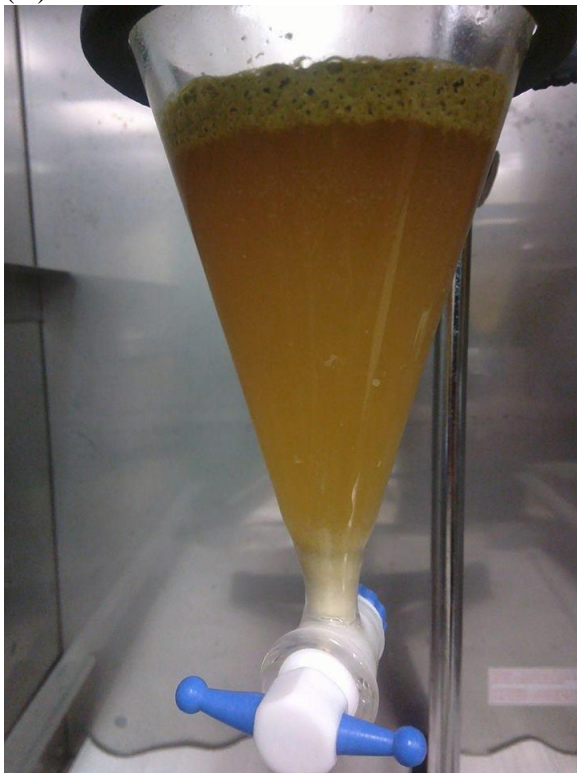
Fig. 1. Flocculation of rumen fluid in separatory funnel. (A) Complete flocculation. Particles form a foamy layer lying on top, and white layer at bottom (mostly protozoa) are free of particles. (B) Incomplete flocculation, showing some particles settling on top of bottom white layer.
