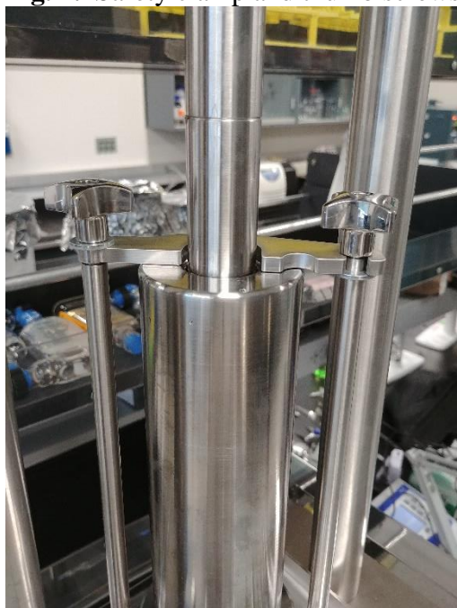
Fig. 4. Safety clamp and thumb screws used to secure cell body
