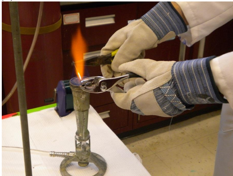
Fig 12. Bending needle of gassing probe. (A) Flaming needle above hub. (B) Bending needle around metal stand.
